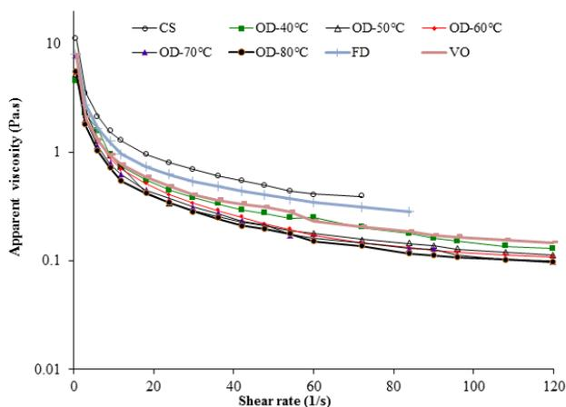
Figure 1. Effect of different drying methods on apparent viscosity of Basil seed gum solution as a function of shear rate; control sample (CS), oven drying (OD), freeze drying (FD), and vacuum oven drying (VO).
