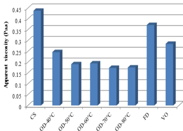
Figure 2. Effect of different drying techniques on apparent viscosity of Basil seed gum (shear rate =  $54 \text{ s}^{-1}$ ); control sample (CS), oven drying (OD), freeze drying (FD), and vacuum oven drying (VO).
